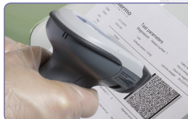
Test parameters can be loaded from a 2D barcode.
