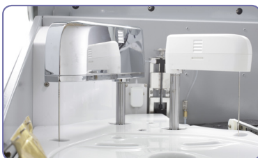
Optional ECM / sample pretreatment unit in its own dispensing arm.
