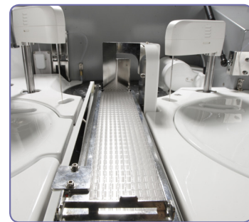
Cuvette loader for 360 cells.
